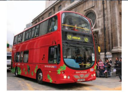
a series arrangement, driving a generator that, in turn, powers the electric motors. Volvo's configuration involves a 5 litre engine (compared to the 9 litre power plant at Euro 4 and 7 litre at Euro 3) in parallel hybrid with the electric ISAM unit.
